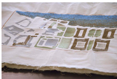
Figure 2: Detail of Aural Fabric and the conductive areas in brown.
